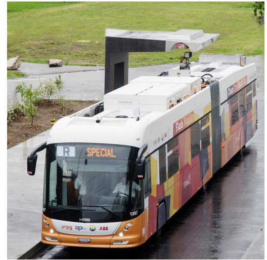
Figure 3: The TOSA electric bus stopped at a charging station in Geneva (Source: Asea Brown Boverly).
