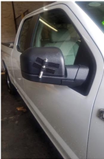
**Figure 2. Example Laser Pointer Attached to Mirror (Source: NYCDOT)**
