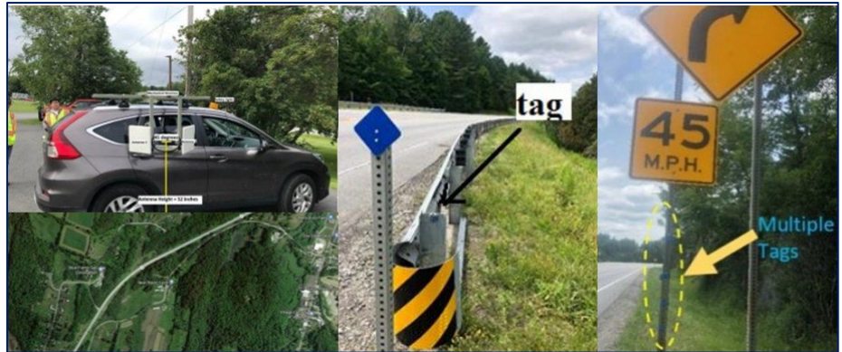
Figure 4: A reader installed on a vehicle continually reads RFID tags affixed to nearby traffic signs and guardrails while the vehicle is in operation, automatically collecting asset data without manual effort (Source: VTRANS).
