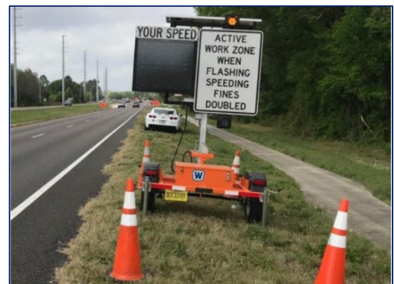
Figure 2: Active Work Zone Awareness Device (AWAD) deployed in a construction zone to protect workers (Source: Florida DOT) Last Modified: May 2025
