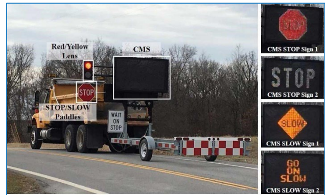
Figure 1. AFAD and CMS Signs Source: MoDOT.
