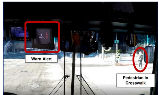
Figure 2: Example bus driver display of pedestrian warning alert as part of the Enhanced Pedestrian Crossing Warning (E-PCW) application in Cleveland, Ohio (Source: FTA).
